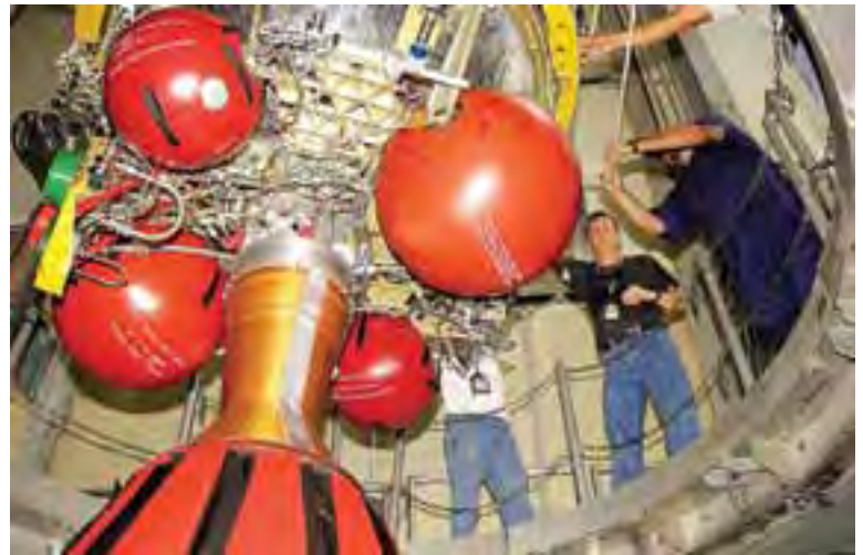
Workers at Launch Complex 17-B, Cape Canaveral Air Force Station, prepare for mating the second stage of the Delta II Heavy rocket to the first stage below. Image Credit: NASA Kennedy Space Center
