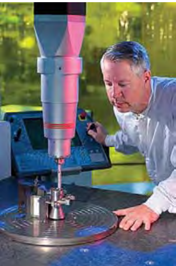
A Pratt & Whitney Rocketdyne technician is taking precise measurements of a small engine thrust chamber. Image Credit: Ross Pakka/Pratt & Whitney Rocketdyne
