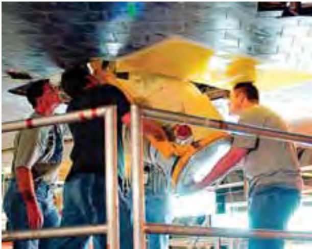
Workers in the Orbiter Processing Facility insert the liquid oxygen feedline for the 17-inch disconnect in the orbiter Discovery. The 17-inch liquid oxygen and liquid hydrogen disconnects provide the propellant feed an interface from the external tank to the orbiter main propulsion system and the three space shuttle main engines. Image Credit: NASA Kennedy Space Center
