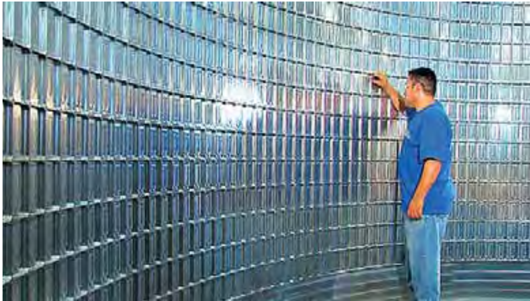
A technician tests a manufactured aluminum panel as part of the Ares I upper stage barrel fabrication. The panels are built by AMRO Manufacturing located in El Monte, California. Image Credit: NASA Marshall Space Flight Center
